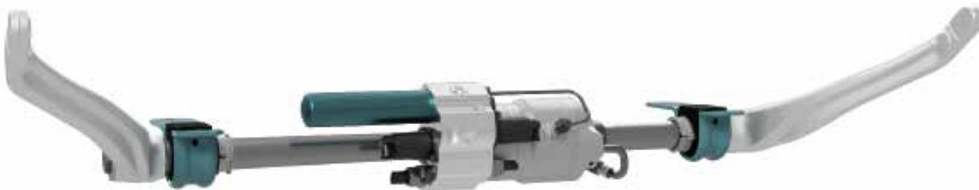
Active roll-control (ARC) systems, implemented to improve vehicle ride comfort and increase wheel articulation while simultaneously providing vehicle roll stiffness and lateral support while cornering, have long been used by automotive manufacturers on their cars, trucks and SUVs. BWI Group has a long history with these systems, developing and manufacturing hydraulic ARC systems in both linear and rotary actuator packages for more than two decades.
